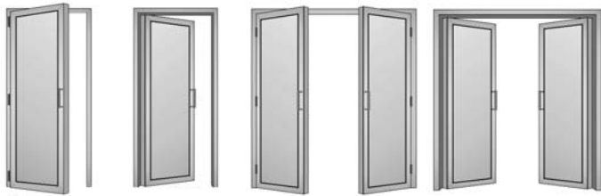
Single door opening outward Single door opening inward Double door opening outward Double door opening inward
